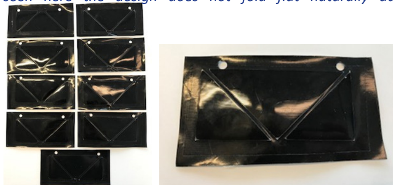
Figure 31: With less than 4mm between faces range of movement is lowered. As seen here the design does not fold flat naturally due to the spacing being too narrow.
