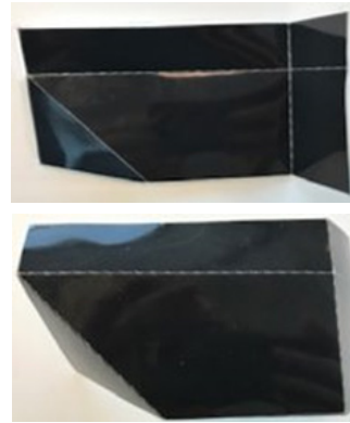
Figures 60-61: Only cut backsheet sample folding forward and sample with only cut frontsheet, folding backwards
