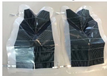
Figure 19 Samples after folding. Left folded by hand, right folded after lines were scored.
