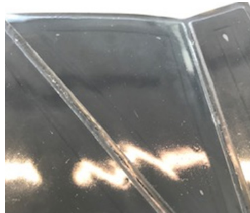
Figure 39: Sample with edge tape (weather proofing) along each edge
