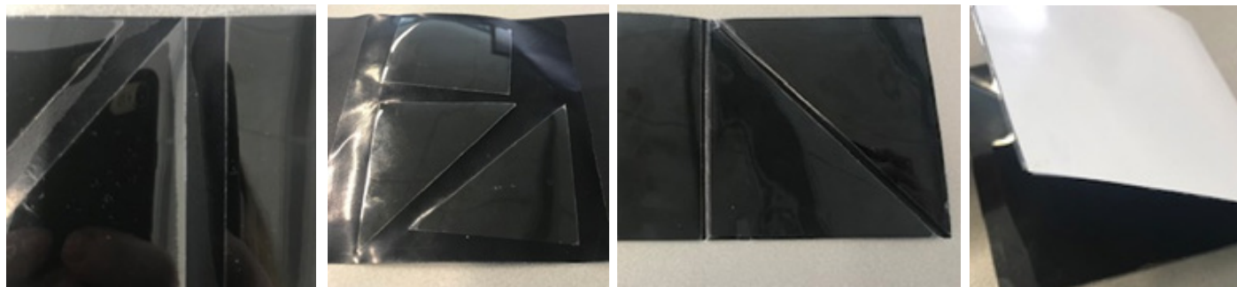
Figure 28: When the encapsulant is not lined up properly peeling can occur, especially in the corners
