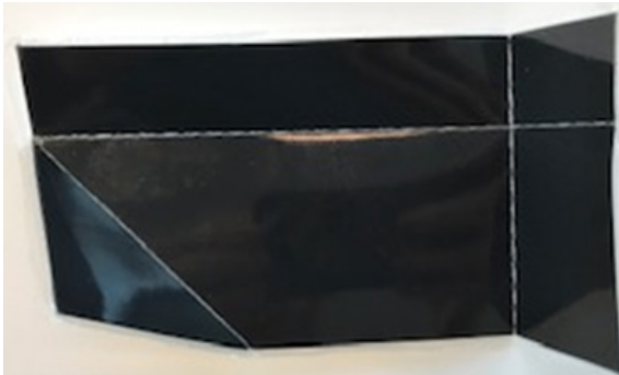
Figure 45-47: Stack of layers with only backsheet cut showing that the sample can fold forward.
