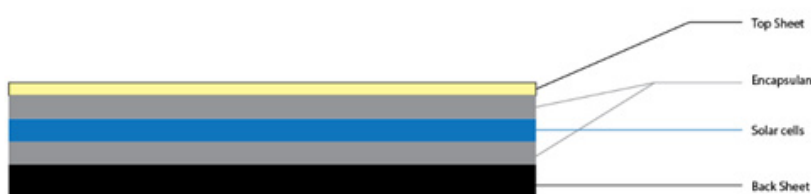
Figure 1: Diagram of the layers on top and below the CIGS cells.
