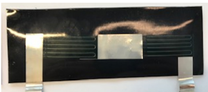
Figure 15: Parallel connections made with tabbing materials, with space between cells
