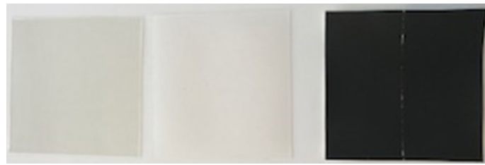
Figure 45-47: Stack of layers with only backsheet cut showing that the sample can fold forward.
