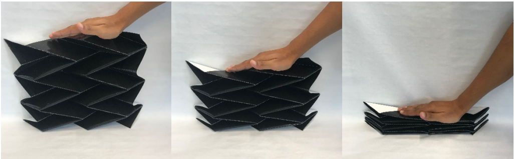
Figures 71-73: Prototype made in final materials. Full scale prototype displays the same flexibility and flat folding abilities.
