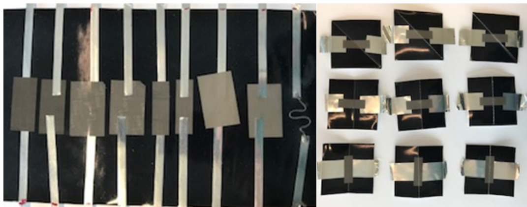
Figure 55 and 56: All alternative tapes tested to see if they can conduct traditional tabbing and further exploration.
