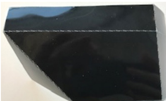
Figure 48-50: Stack of layers with only frontsheet cut showing that the sample can fold backwards.
